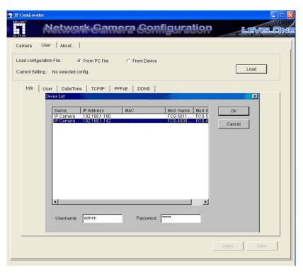
After loading, you can get configuration from PC files or devices. IP CamLocator displays the sub folders including Info, User, Date Time, TCP/IP, PPPoE and DDNS.
